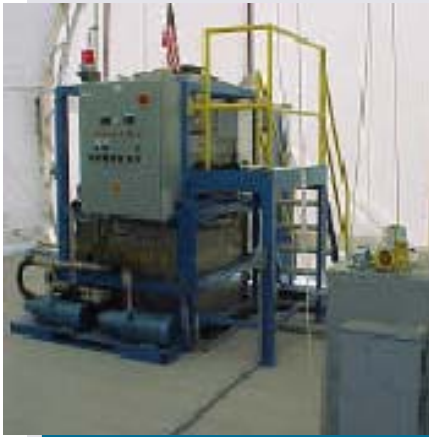
Ciba® ALCOTECH® DWU polymer makedown unit in operation at Conner Creek project
