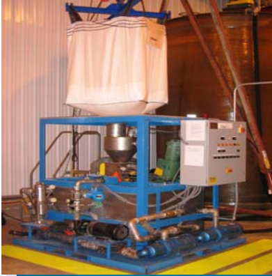
Ciba® ALCOTECH® DWU polymer makedown unit in operation at Fox River project
